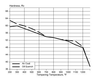
Test samples 1" round x 2" long were hardened by air and oil quenching from 1725°F and tempered at the indicated temperaures. Resulting hardness is shown above.
