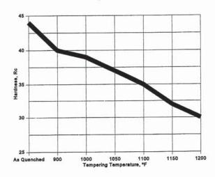
4-inch cubes, quenched in oil from 1575°F, tempered 2 hours at indicated temperatures.
